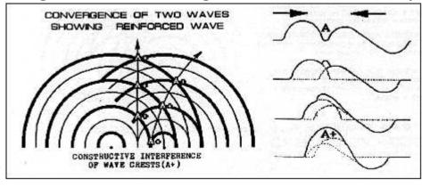
waves are taller and reinforced. Each model of the AcoustiCoil creates a specific desired amount of interference within the instrument.
